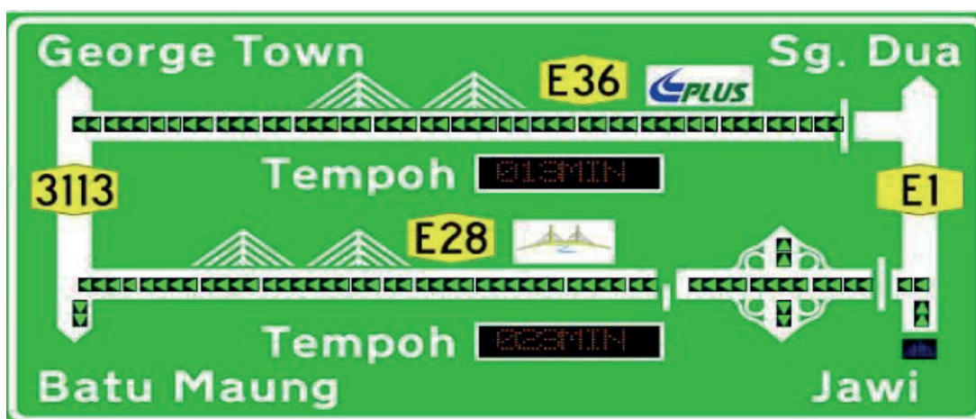
Figure 46. VMS Application in Malaysian (Source: Malaysian ITS Blueprint (2019-2023), 2019)
